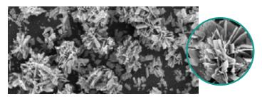
An example of zinc borate with a platy open particle structure. It could reduce powder flowability and bulk density—potentially affecting process handling and distribution.
