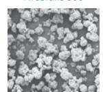
The more rounded particle shape of U.S. Borax *Firebrake* zinc borate products promotes consistent powder flow, process handling, and distribution in the product.
