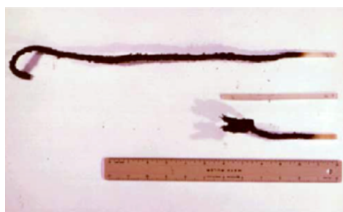
Figure 4: Intumescent char of epoxy. Top sample contains Firebrake ZB and dechlorane plus.
