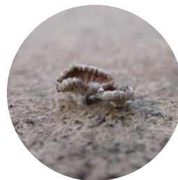
Field tests show decay fungi thriving on untreated WPCs.
