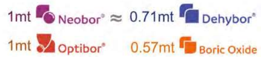
Figure 7: Comparison of hydrated and anhydrous borates for glass on B 2 O 3 basis.
