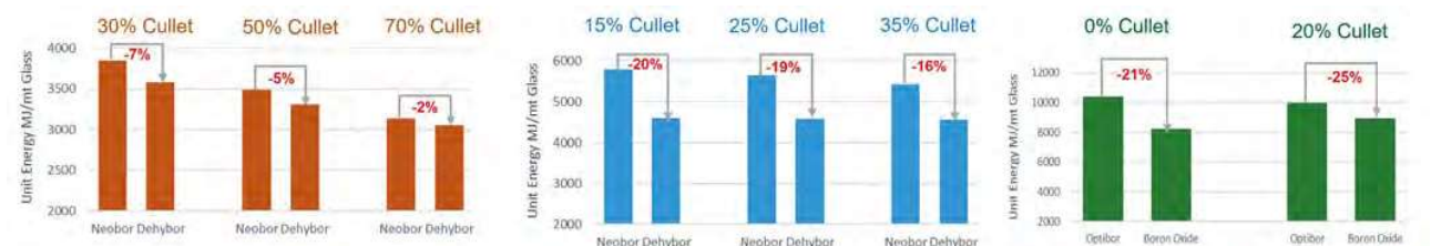
Figure 5: Unit energy reduction due to increased pull rate for (a) Glass wool (b) Type 1 pharmaceutical glass (c) TFT glass.
