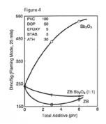
In the presence of alumina trihydrate (ATH), *Firebrake* ZB reduces smoke effectively, even when used with antimony trioxide. In the absence of ATH, a high ratio of *Firebrake* ZB to antimony trioxide is recommended for low smoke formulations.
