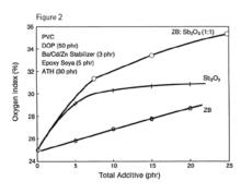
In the presence of alumina trihydrate (ATH), there is a dramatic synergism between *Firebrake* ZB and antimony trioxide. This synergism is observed at a total loading as low as 3 phr.
