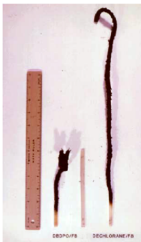
Figure 4 Intumescent Char of Epoxy Containing Firebrake ZB and Dechlorane Plus (sample on the right)
